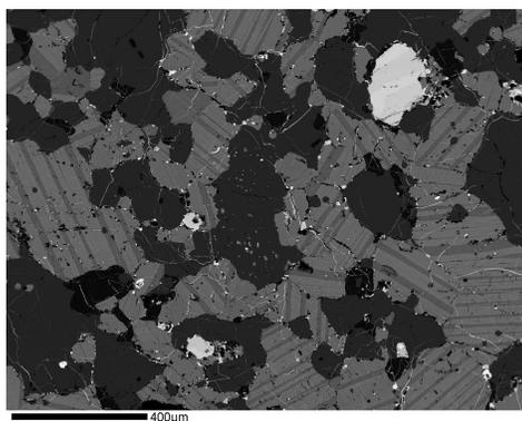
**Figure 3.** Back-scattered electron image, showing exsolved pigeonite grains (with prominent broad, parallel clinopyroxene exsolution lamellae in host orthopyroxene), calcic plagioclase (dark gray), silica polymorph (black) and Fe-Ti-Cr oxides (lightest gray).
